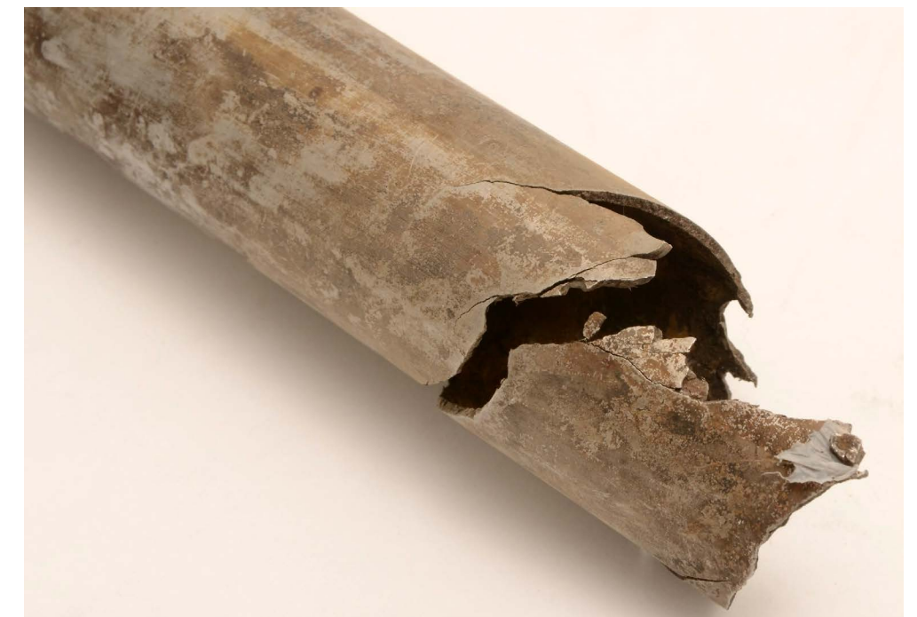
Fig. 3 Stress corrosion cracking of 304L
