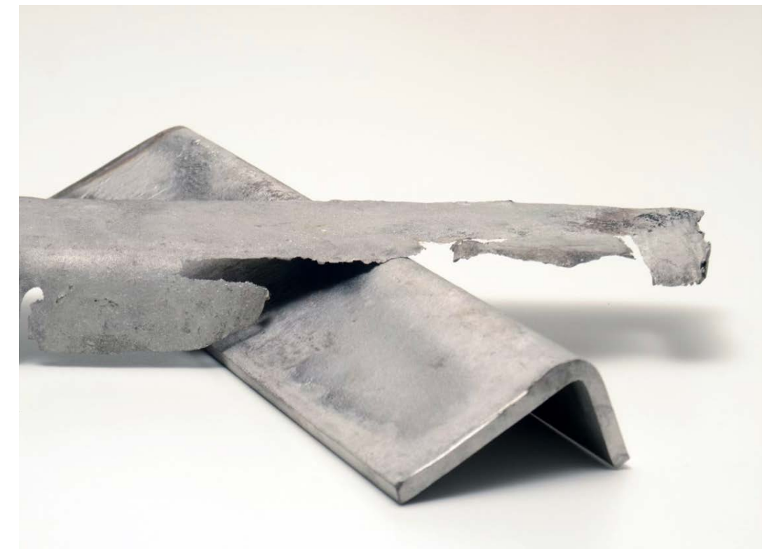
Fig 1 Alloy 825 corroded in H_2SO_4 when exposed to extreme temperature.
